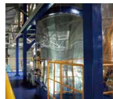
Atomization mode: Rotary atomizer Drying chamber diameter: φ3400 mm Water evaporation capacity: 86 kg/h
