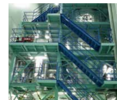
Atomization mode: Rotary atomizer Drying chamber diameter: φ4000 mm Water evaporation capacity: 100 kg/h
