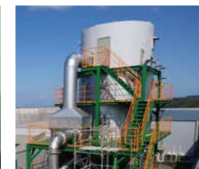
Atomization mode: Rotary atomizer Drying chamber diameter: φ5000 mm Liquid material processing capacity: 500 kg/h
